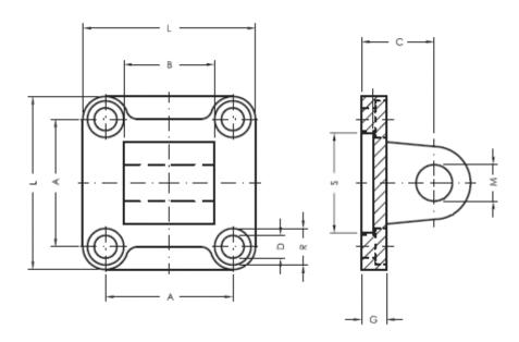
R = 18 = 89.0 Α В = 60 Countersunk screw = 41 Cylinder size = 100 = 11.0 D G = 14 L = 115 = 20 Μ
